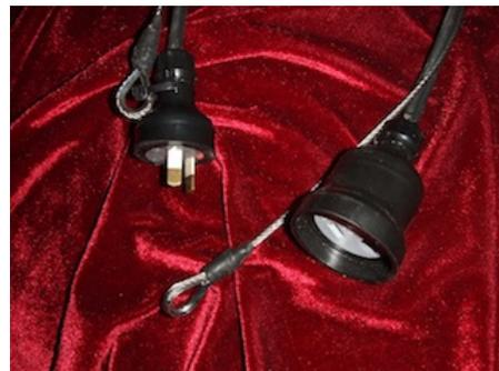
**2. Hang all the strings up before fitting any globes.** Attach using the stainless steel eyelet or guy wire provided, never attach directly to the electrical cable. To join the 16m festoon strings together, use the small "D" shackle provided, this will ensure the guy wire is taking the strain and that there is no strain on the plug & socket connection.
